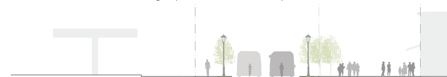
Limited Access Framework Section A-A Chicago Avenue (Looking North) Pedestrian, bicycle and transit mall, with access for emergency, maintenance and delivery vehicles.
